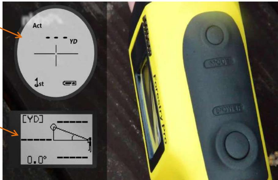
Press ON for a second and the LCD becomes visible. Then press the **MODE** button and the LCD display will open (see below). The external LCD display is used to show results and the internal one (viewed through the eye piece) is used to check the settings. By default, the device is set to measure the Linear Distances, however you can change that setting.
