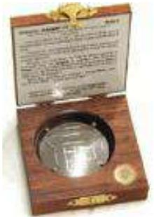
1. Hold the densitometer far enough away from your body so that your head is just outside the grid (30–45 cm away), **at 0.8 m above the ground** (i.e. at waist height). Use a measuring stick to get the correct height. Keep the densitometer instrument level, as indicated by the round level in the lower right hand corner.
