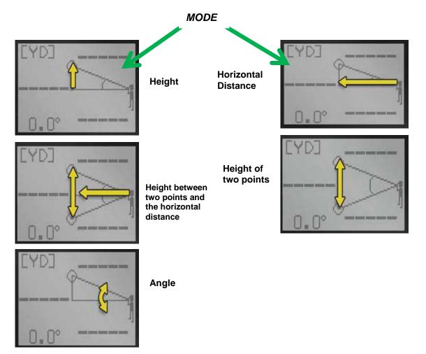
2. To change the **Units of Measurement** (metres [M], feet [FT]) from the default **[YD]** or from other unit that you are not going to use, press and hold the **MODE** button for a couple of seconds and internal display will change to the new priority mode. Press and hold again and again until you have reached the unit you are going to use.
