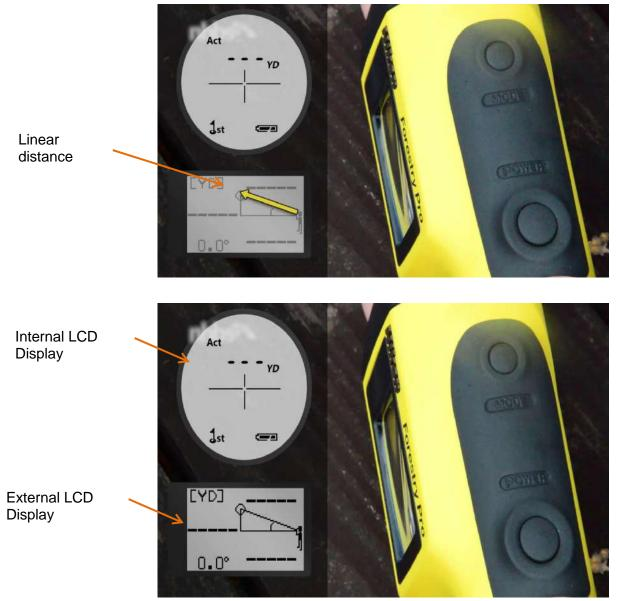
Press ON for a second and the LCD becomes visible. Then press the **MODE** button and the LCD display will open (see below). The external LCD display is used to show results and the internal one (viewed through the eye piece) is used to check the settings. By default, the device is set to measure the Linear Distances, however you can change that setting.
